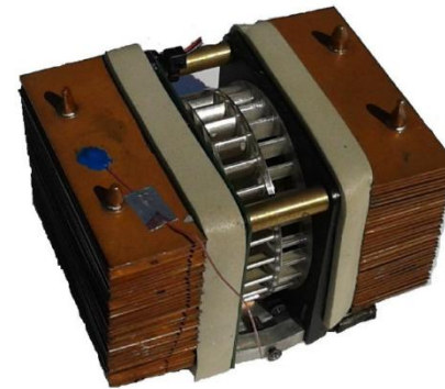
High performance cooler, R_t = 0.18 \text{ } ^\circ\text{W}
